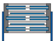
METALLIZED FILM & DOUBLE SIDE METALLIZED DESIGN (INTERNAL DESIGN)
